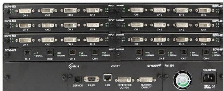
Figure 1-2 Rear panel of OMM-1000
