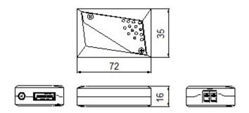
Note: The transmitter, DPFX-100-T and the receiver, DPFX-100-R have the same mechanical dimensions
