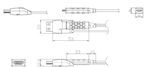
Dimensions (L\*W\*H) Tx: 65 x 20 x 11.5mm Rx: 50 x 20 x 10.4mm
